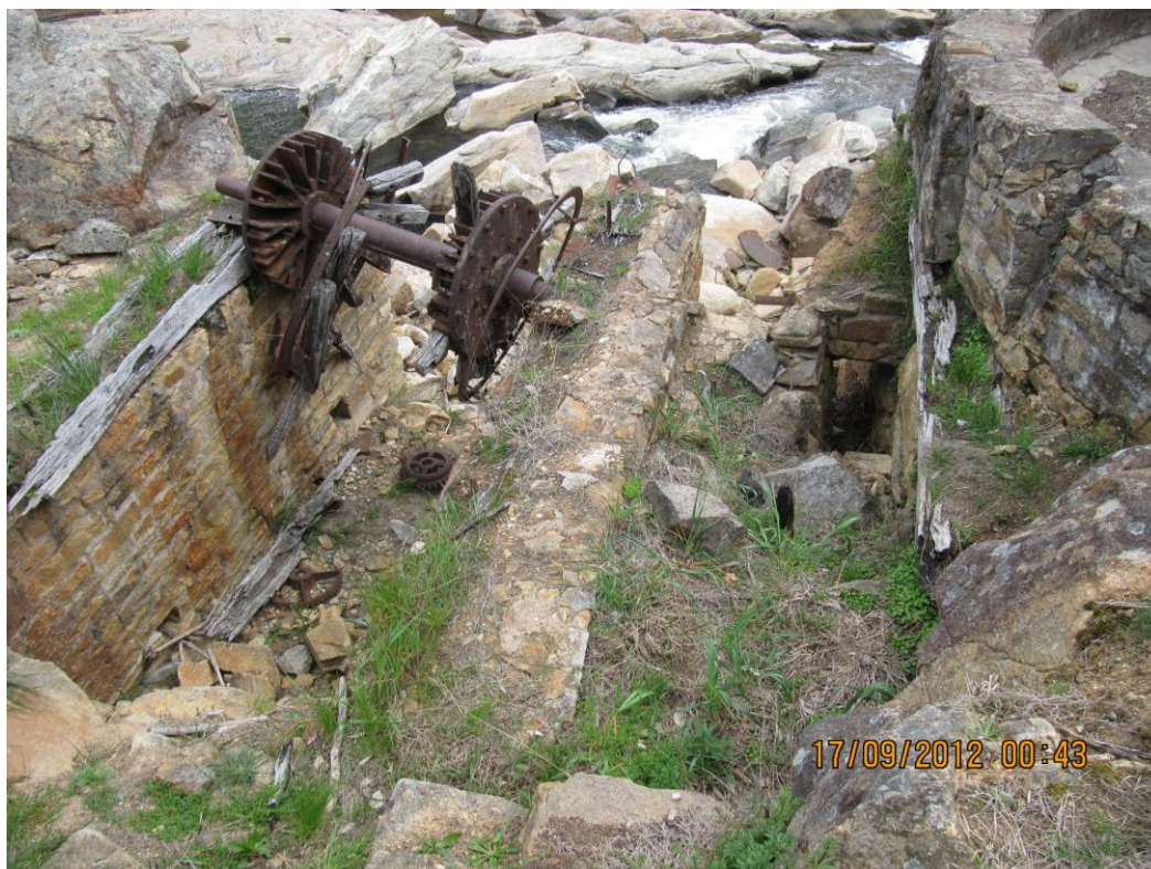
Hub of 26ft [7.9m] lower water wheel
