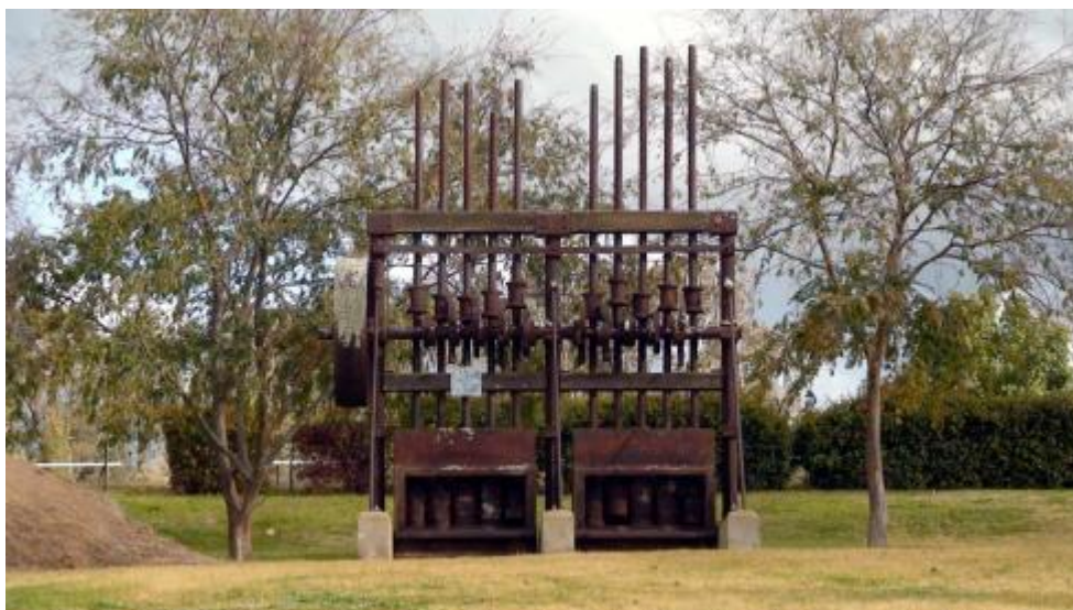
2 stands of 5-head stamper batteries Harrietville Museum
