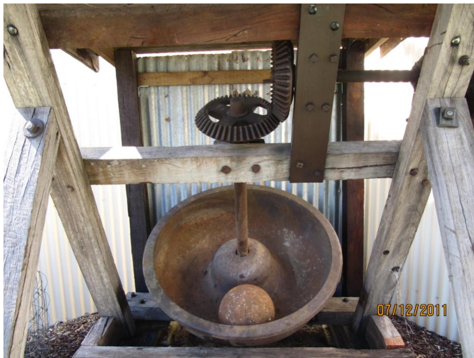
Berdan Pan with cast iron ball Harrietville Museum
