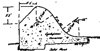
Fig. 18.—Typical Section of Bywash Weir—Type K.
