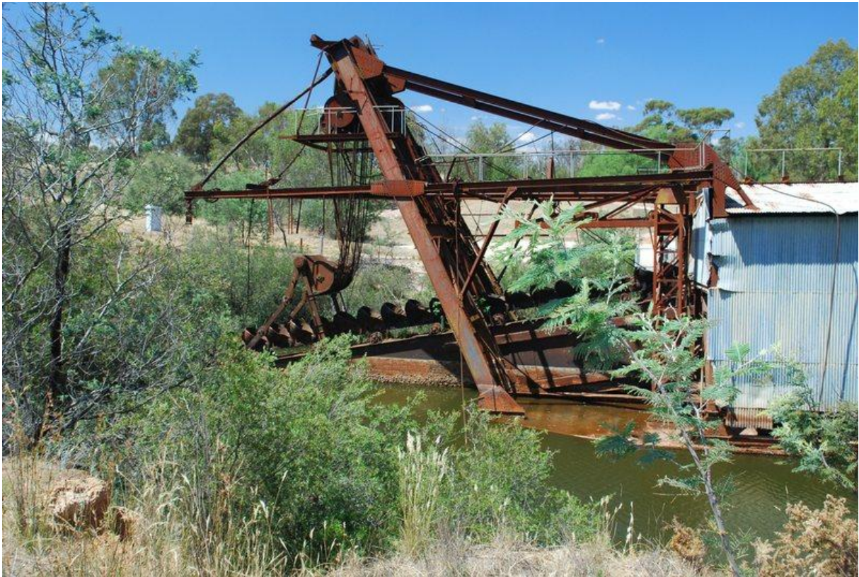
Figure 7: Bow end of the dredge viewed from north, showing the inclined fore-gantry, sitting on the partly submerged front forks of the pontoon. Also shows part of bucket ladder, and the supporting cables and pulleys, (now hanging slack). (Photo from Heritage Victoria website.)
