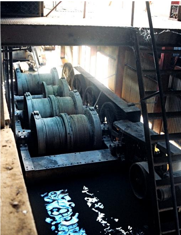
Figure 11: The linked winches for mooring and manoeuvring the dredge, on the semi-submerged deck beneath the control room, here viewed from stern end. (Photo by C. Doring, 1994)
