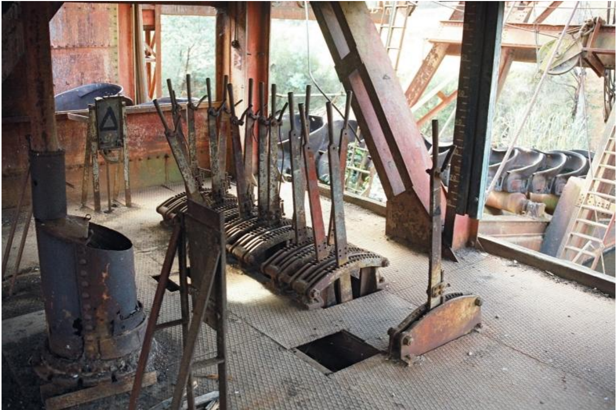
Figure 12: Levers in the control room, mechanically controlling clutches or brakes on the winch drums below. The open front wall normally had windows and cgi cladding, stolen here but since replaced. At left is a small stove for warmth – a rare concession to operator comfort. (Photo by C. Doring, 1994)
