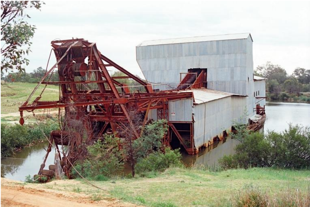
Figure 2: General view of the dredge, seen from East, with bow end in foreground. Note the upper end of the inclined bucket ladder emerging from an opening in the tall central section of the superstructure, and the lower end with buckets at bottom left corner of the photo. Also in foreground is the fore-gantry frame with pulleys and steel cables to raise or lower this end of the bucket ladder. (Photo C. Doring 1994)
