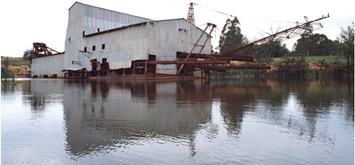
Figure 3: General view of the dredge from NW, showing the bow end at far left and the stern end at centre, with gravel-disposal chutes protruding from the stern at right. . (Photo by C. Doring 1994.)
