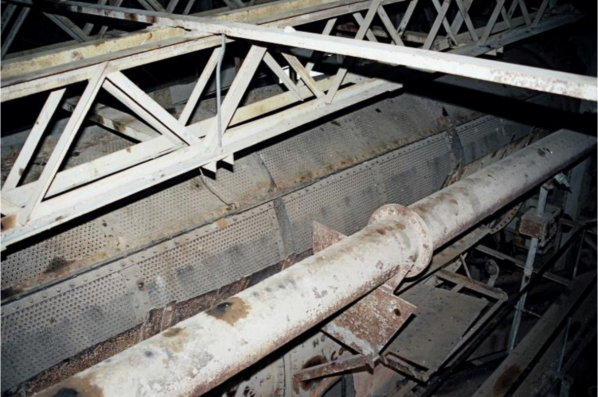
Figure 13: Part of the cylindrical sidewall of the rotary screen, made of curved steel plates with hundreds of small holes. The rest of the screen is difficult to see. (Photo by C. Doring, 1994)
