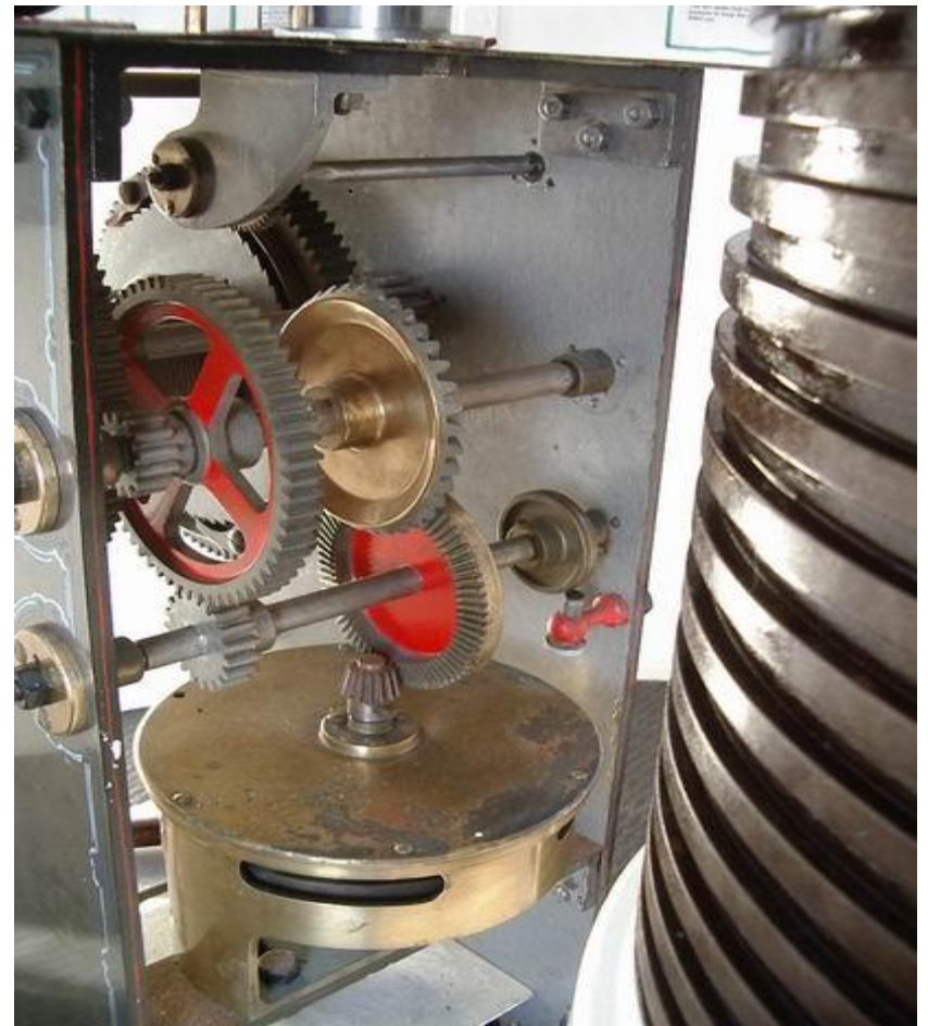
'Clock' – clockwork motor similar to the replacement one that was installed in 1926 The governor is at the bottom and the adjusting screw of the pedestal can be seen on the right of the picture
