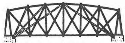
Figure 10 The McCallum truss was popular in America but only two sets were built in New South Wales, at Cowra in 1870 and at Casino in 1874. The untidy arrangement made construction difficult and maintenance was not an easy task.
