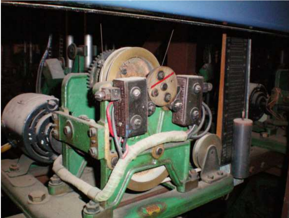
One of the Barometer Indicator Drive Units in the Eagle Farm Racing Museum
