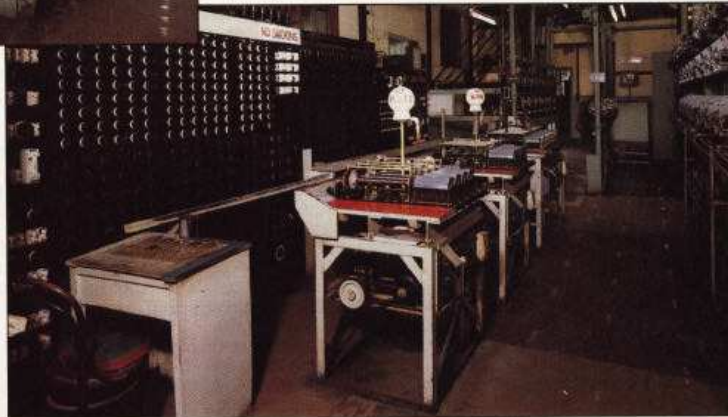
The tote room coordinates the accumulation and display of the pools and contains the machine which calculates the winning odds. The "odds machine", with its array of local aggregators (above), stands in the far distance
