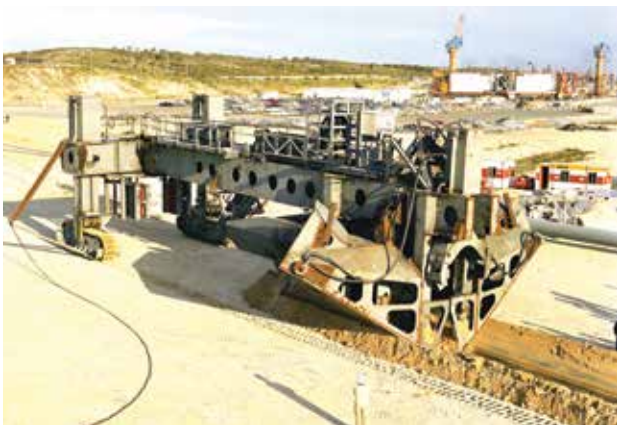
Figure 5: The 380 tonne subsea plough underwent a series of land tests at Jervoise Bay, south of Perth
