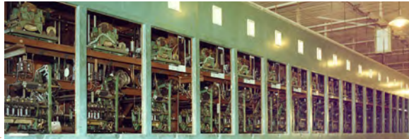
50 indicator drives and adding machines formed the 1948 Eagle Farm totalisator – 24 for win bets backed by 24 for place bets plus two for the grand totals
