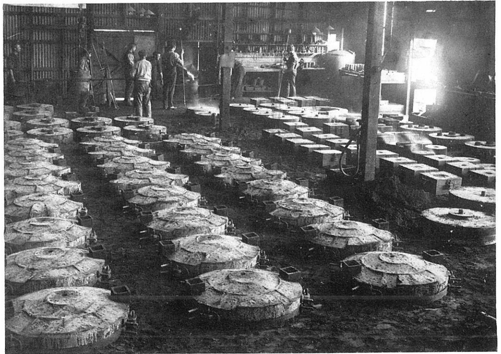
Tank end moulds, ready to pour, 1910
